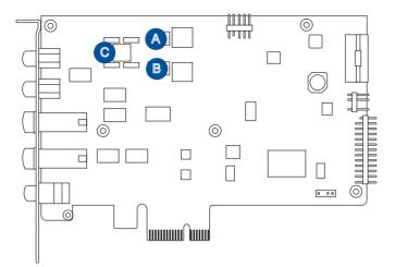
There are three swappable op-amp sockets in Essence STX II. Changing the op-amps affects the tonal characteristics of the RCA outputs, while changing A and B affects the tonal characteristics of the 6.3mm (1/4") headphone output.
