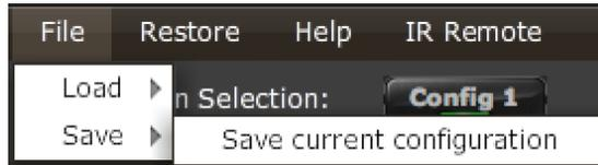
To load a configuration, first select the configuration preset that you wish to load into. Then drop down the File menu, select **Load**, and then **Load configuration to current slot**.
