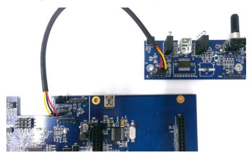
2) Front panel connectivity for miniDSP 2x8 PCB v1.1 and all miniDSP 8x8 (Most common)
