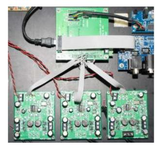
Example 2: Connection between miniSHARC and 3 curryman DAC using ribbon cable
