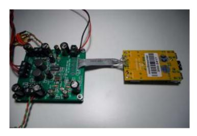
Example 1 : Connection between miniSTREAMER and curryman DAC using ribbon cable
